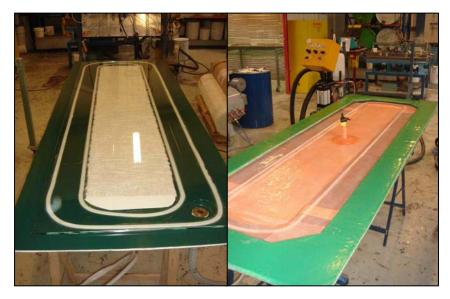
Fig. 1 RTM light / ECO and CCBM linear tool.
